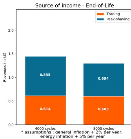
In the French market, peak-shaving provides a slightly higher share of savings, so a moderate cycling strategy is needed, as confirmed by the currently slightly higher internal rate of return. Even if moderate cycling generates less savings at the beginning of life, the difference in savings over the lifespan is compensated with a positive IRR of 0.6%, compared to 0.5% for intense cycling.
